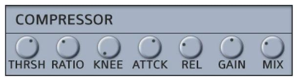
All of the layers are summed up into a Compressor, before reaching the Main Filter. The Compressor can be used to tame or squash a drum, depending on how hard you push it. A dry/wet mix control is provided for getting the right balance. Here's a rundown of the Compressors controls and what they do:
