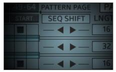
Click the box above the editing controls to display the Sequence Shift functions. These arrows will move a sequence lane forward or backward, step by step. This can be very convenient for times when an entire row of steps need to be shifted over slightly.
