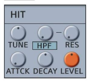
The next stage of the Drum Editor is the Hit Layer. This layer adds extra top end to the drum sound. This can give the drum more of an initial 'attack'. The Hit layer can be Tuned separately (+ or - 1 octave). It also has it's own Attack and Decay settings. The Attack is very short, and is meant to dull the sound if it is too sharp, removing some of the transient.
