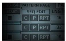
To the right of each sequencer's grid are 3 buttons for editing the sequence. **C** is for **Copy**. Use this to copy the steps of one sequence lane to another. This will copy all 64 steps including the Accent and Flams of
