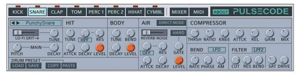
The top half of PulseCode's interface is dedicated to sound design of the drums, as well as audio and midi related functions. The bottom half is for the Pattern Sequencer and all of it's related functions. In this section we will look at the top half, specifically the Drum Engines.
