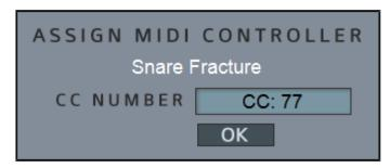
Each parameter can be assigned to midi control. This includes all knobs and sliders and most buttons and switches. Midi assignment can be done right from the GUI. Just right-click on a parameter and a pop-up screen will appear. Move the desired control on your Midi controller and it will appear in the Midi CC display. Alternatively, you can click on this display to bring up a list of Midi CCs for manual selection. Click 'Ok' when finished.
