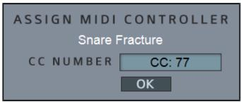
Each parameter can be assigned to midi control. This includes all knobs and sliders and most buttons and switches. Midi assignment can be done right from the GUI. Just right-click on a parameter and a pop-up screen will appear. Move the desired control on your Midi controller and it will appear in the Midi CC display. Alternatively, you can click on this display to bring up a list of Midi CCs for manual selection. Click 'Ok' when finished. \*The Midi Learn section also supports NRPN
