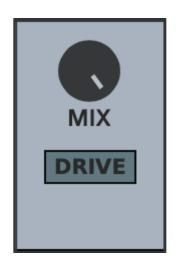
The Mix control mixes between the dry signal and the signal fully affected by the Tone section. The Drive switch beneath it determines if the dry signal will respond to the Input Drive control. For example, if Drive is switched on, both the dry and wet signals will respond to the Input Drive control. This will have the effect of equal loudness in the mix. If this button is switched off, the dry signal is completely dry, most likely resulting in a much lower dry signal.
