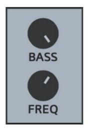
The Bass control acts as a bass booster, increasing the low-end frequency set by the Freq control beneath it, which ranges from 30-95 Hz.
