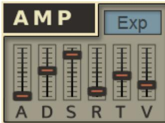
The Amplitude Envelope controls the overall volume when a key is triggered. This envelope can control the filter as well if assigned to it.
