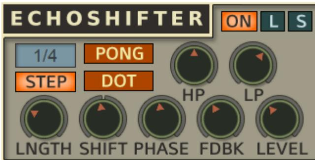
The EchoShifter is a hybrid pitch-shifting dub delay unit. It is capable of some very interesting effects, from detuned space echoes to otherworldly atmospheres. The feedback, when cranked up, can become an infinitely evolving sound source. Here is an overview of what each control does.
