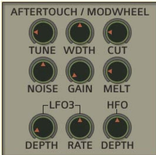
If your MIDI Controller allows it, Aftertouch will send MIDI data when pressure is applied to it's keyboard while notes are being held. This means that if aftertouch is routed to filter cutoff, applying pressure to the keys will open up or close the filter, depending on how this is set up.
