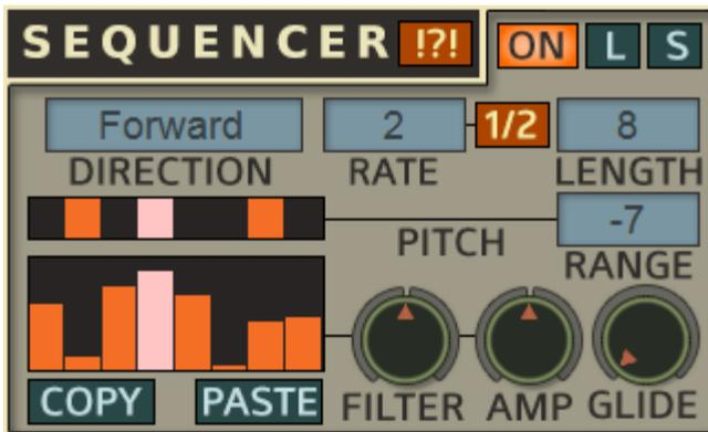
Phonoc's Sequencer works like a modulator. Rather than triggering MIDI notes, it will modulate the pitch, filter cutoff and amplitude in steps. This allows the Sequencer to work alongside the Arpeggiator. The arp controls the MIDI notes, while the sequencer accents the pitch and velocity. The sequencer can be used by itself if desired for things like rhythmically modulated pads.
