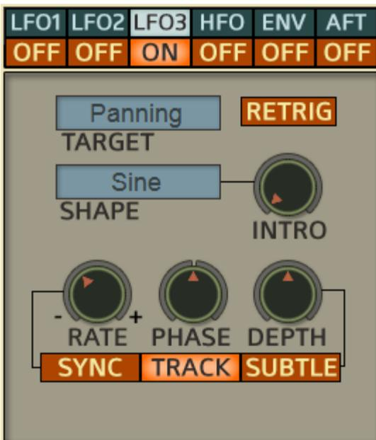
Phonec2 has three LFOs (Low Frequency Oscillators) that can modulate various parameters such as pitch, filter cutoff, panning, etc.
